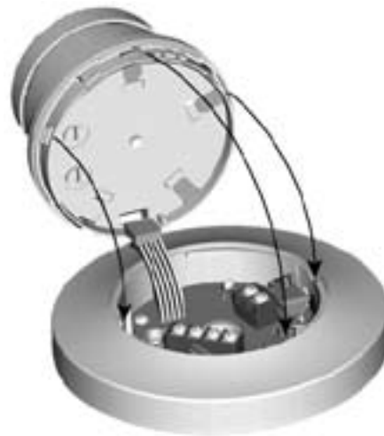
Figure 5: Installing Filtrex detector into base:
